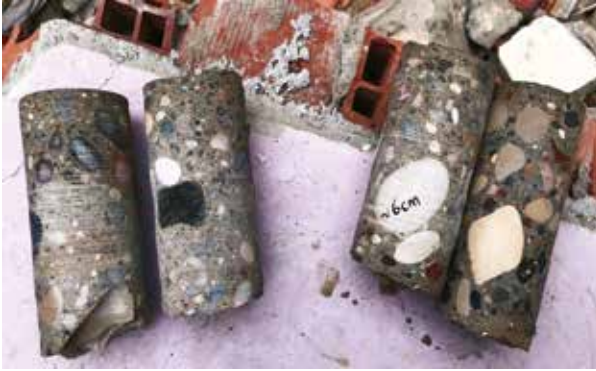
Above: Evidence of the non-compliant reinforced concrete used in the construct of damaged buildings.
