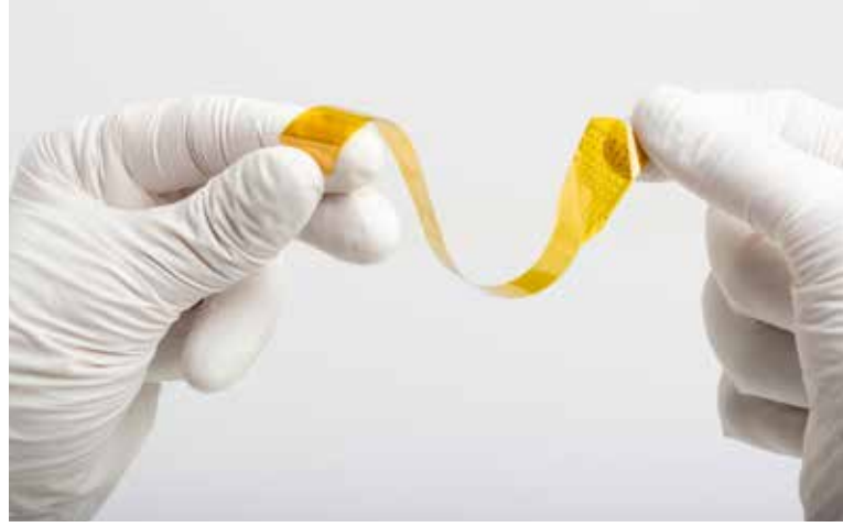
The Layer 7 cortical interface, Precision Neuroscience's thin film microelectrode array.
